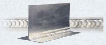
Base metal: AIMg 3 Sheet thickness: 0.6 mm Filler metal: AIMg 5, ø 1.2 mm Shielding gas: Argon
